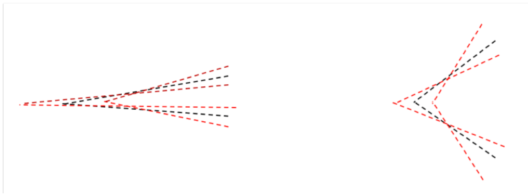
Figure 5.8: Effect of opening angle on Vertex Resolution
