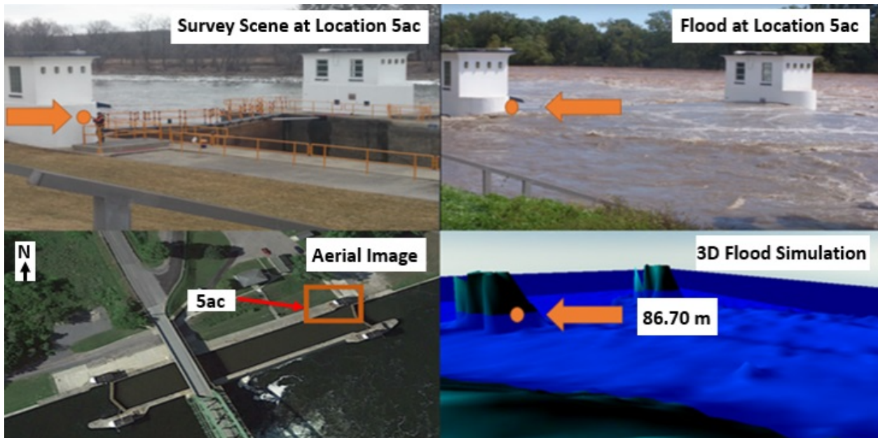
Figure 2: Lock Station 12 where flood simulation and GPS measurements were taken. (A): location 5ac during the GPS survey; (B): image of the flooding occurring at location 5ac (YouTube, 2011); (C): aerial view of flood location 5ac; (D): 3D simulated flood model of location 5ac.
