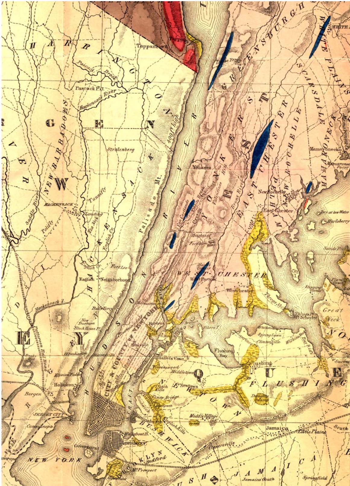
Figure 3 – A portion of the first geological map of New York County and vicinity showing the extent of “Primitive” limestone (blue lenses) and crystalline rocks (pink). (From Mather, 1843.)
