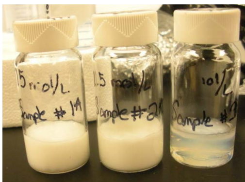
Fig. 1: NIPA gels as prepared in 20 mL vials. The higher molar concentration are more opaque than the lower molar concentrations.
