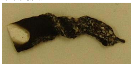
Figure 3: PS, PMMA, Bromine burned.
