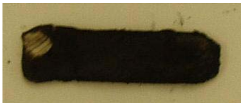
Figure 2: PS, PMMA and Clay burned
