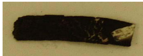
Figure 4: PS, PMMA, Bromine and Clay burned.
