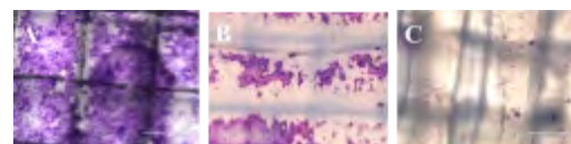
Figure 2: E. coli Biofilms stained with Crystal Violet 22 hours after plating on Ultimaker samples. A: Control, B: 0.01M PLA-AgNO 3 , C: 0.1M PLA-AgNO 3
