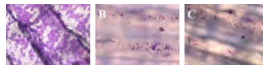
Figure 3: S. aureus Biofilms stained with Crystal Violet 48 hours after plating on Ultimaker samples. A: Control, B: 0.01M PLA-AgNO 3 , C: 0.1M PLA-AgNO 3
