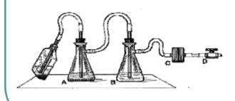
A suction flask is used to collect the contaminated fluids into a suitable decontamination solution. A second flask serves as a fluid overflow collection vessel and an in-line HEPA filter is used to protect the vacuum system from aerosolized microorganisms.
